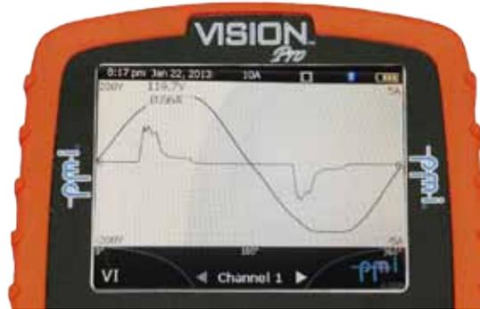
Figure 2. Output from a 23W Compact Fluorescent Lamp
