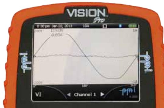
Figure 3. Output from 2.5W Light Emitting Diode Lamp
